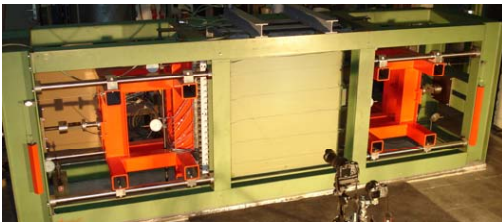
Figure 5. Apparatus for plain strain testing of reinforced soil.
