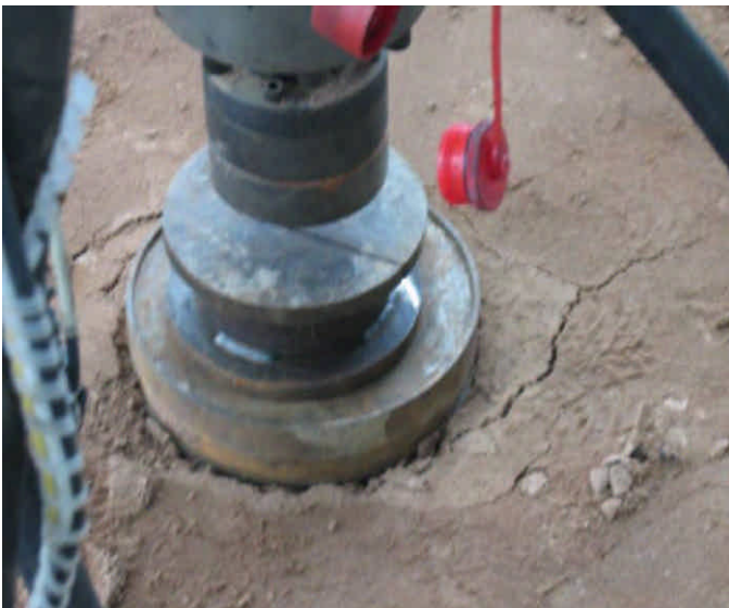
Figure 7: Cracks at the sub base surface
